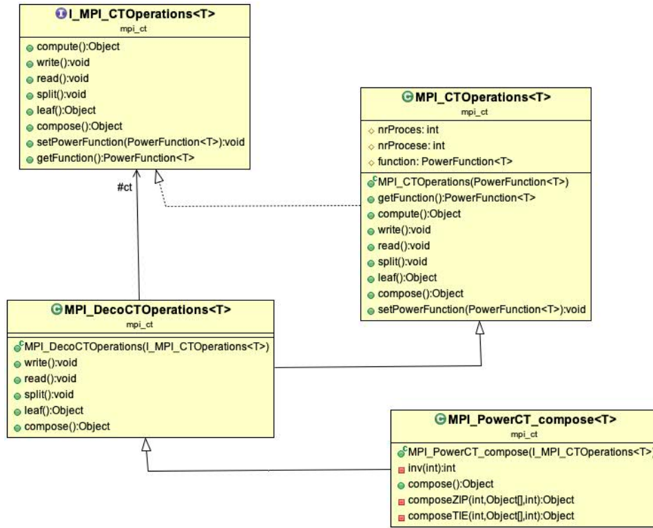
Figure 6: Implementation details of some of the classes involved in the definition of MPI execution.
