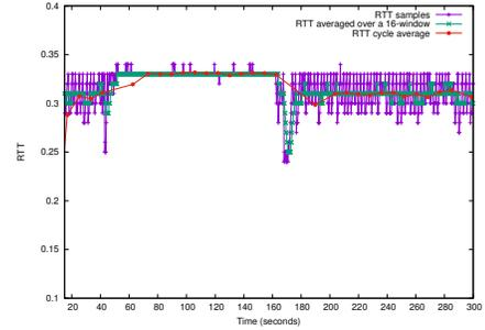
Fig. 2. The two-stages smoothing performed on RTT samples
