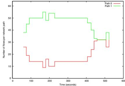
Fig. 4. The number of multihoming flows mapped on each path by the multihoming routing algorithm; DropTail queuing and 100Mbps capacity
