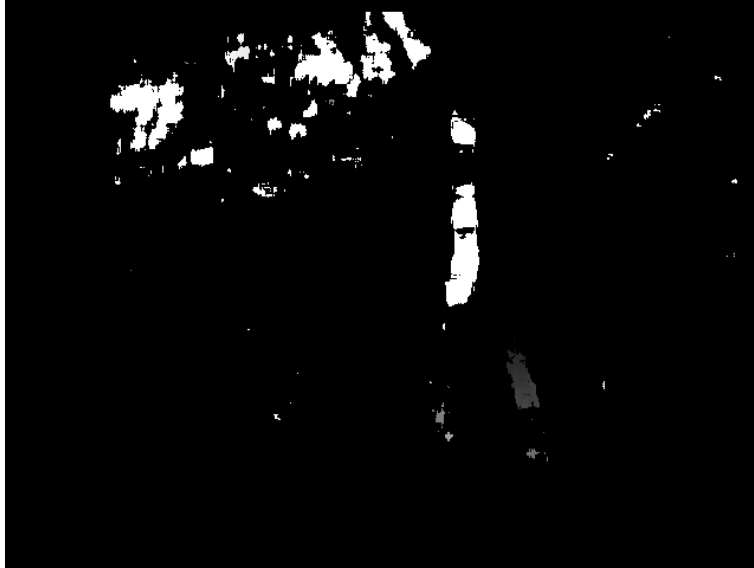
FIGURE 4. The disparity map of the two images in Fig. 2 and Fig. 3
