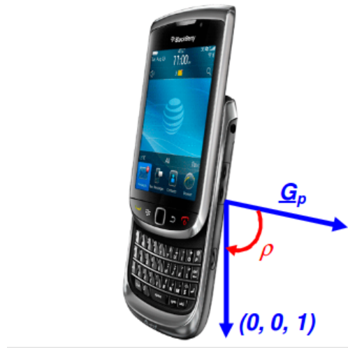
FIGURE 2. Accelerometer axis orientation, after [13]
