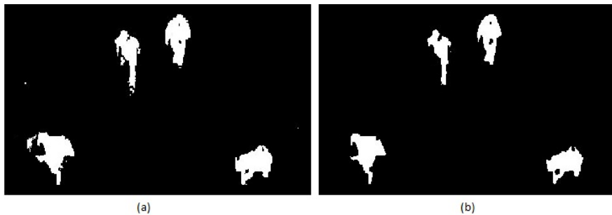
FIGURE 3. Binary image(a), Eroded image(b).
