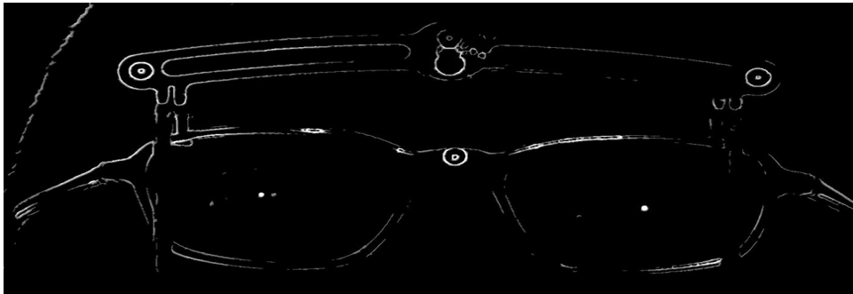
FIGURE 4. Final preprocessing step: Canny Edge Detection and Closing
