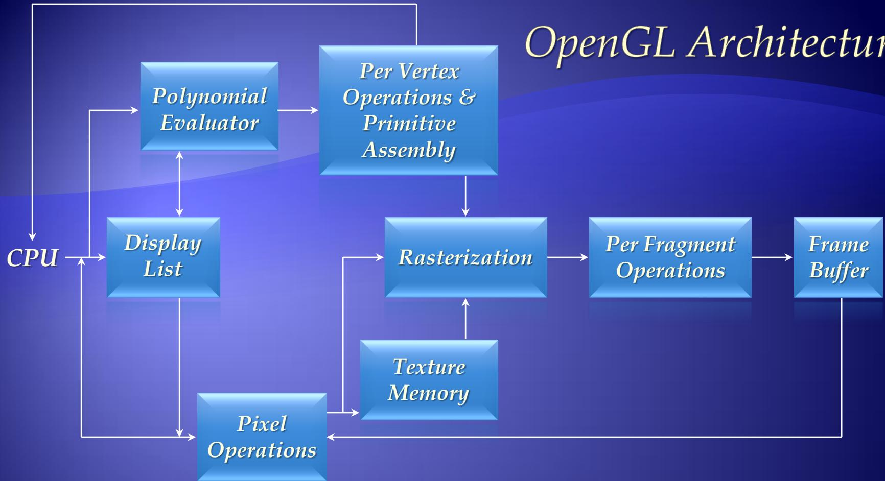
This is the most important diagram you will see today, representing the flow of graphical information, as it is processed from CPU to the frame buffer. There are two pipelines of data flow. The upper pipeline is for geometric, vertex-based primitives. The lower pipeline is for pixel-based, image primitives. Texturing combines the two types of primitives together. There is a pull-out poster in the back of the OpenGL Reference Manual ("Blue Book"), which shows this diagram in more detail.
