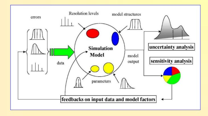
Ideal scheme of a possibly sampling-based sensitivity analysis. Uncertainty arising from different sources — errors in the data, parameter estimation procedure, alternative model structures — are propagated through the model for uncertainty analysis and their relative importance is quantified via sensitivity analysis.
