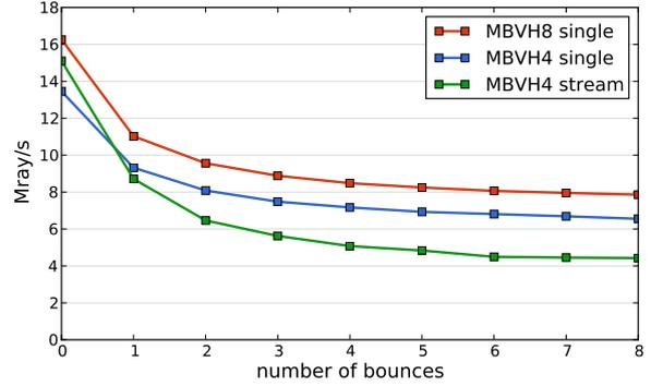
**Figure 2:**  $N$ -bounce diffuse path tracing performance (including primary rays and shading) for the SAN MIGUEL scene for the fastest three methods. MBVH8 single traversal (our proposed method) outperforms both MBVH4 single traversal (the Embree method) and MBVH4 stream traversal (MBVH RS).
